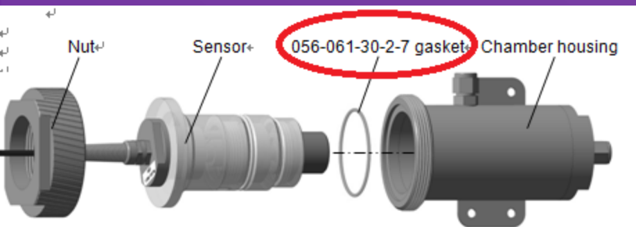
Figure 4.2 – Sensor mounting in the chamber
